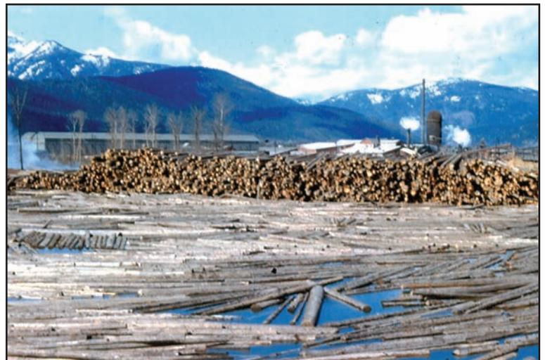
*Mill pond ~ decked logs are rolled into pond as needed*
